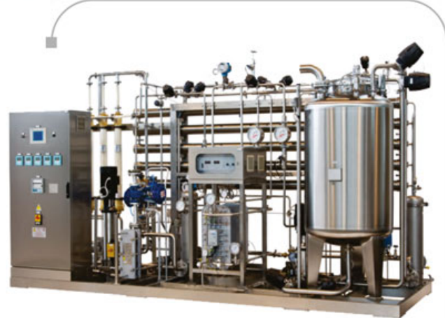
2000 LPH PURIFIED WATER GENERATION SYSTEM
